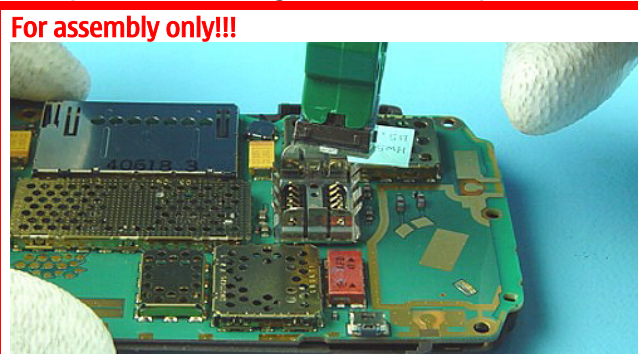
20) For Camera Module assembly use the backside of the Camera removal tool SS-15 and mind the three guide pins.
