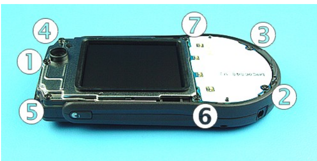
7) Unscrew the seven Torx Plus® size 6 screws. For assembly, the reverse order and a torque driver with a torque of 25Ncm has to be used.
