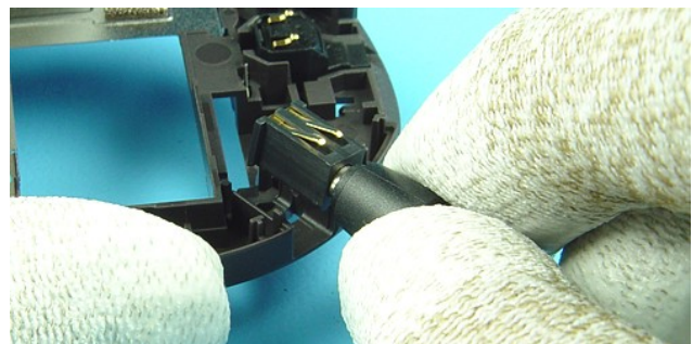
24) Remove the DC Jack by using a DC Plug .
