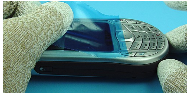
2) Protect the window with a protective film.
