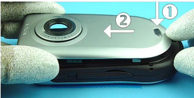
3) To remove the Back Cover press the release button.
