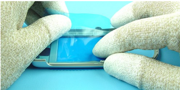
5) Protect the inner side of the window with a protective film.
