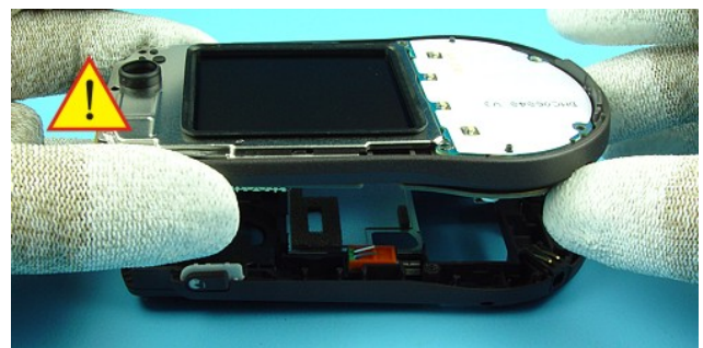
8) Lift up both parts, the UI Frame Assy and the Engine Module simultaneously from the Chassis Audio Assy to prevent mechanical stress from the LCD connector.
