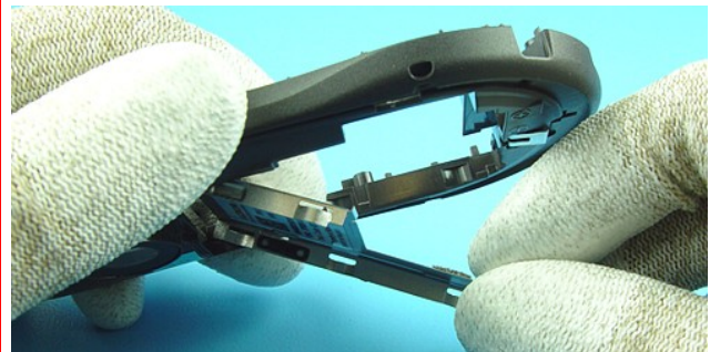
30) Remove the Card Plate incl. Ground Gasket .
